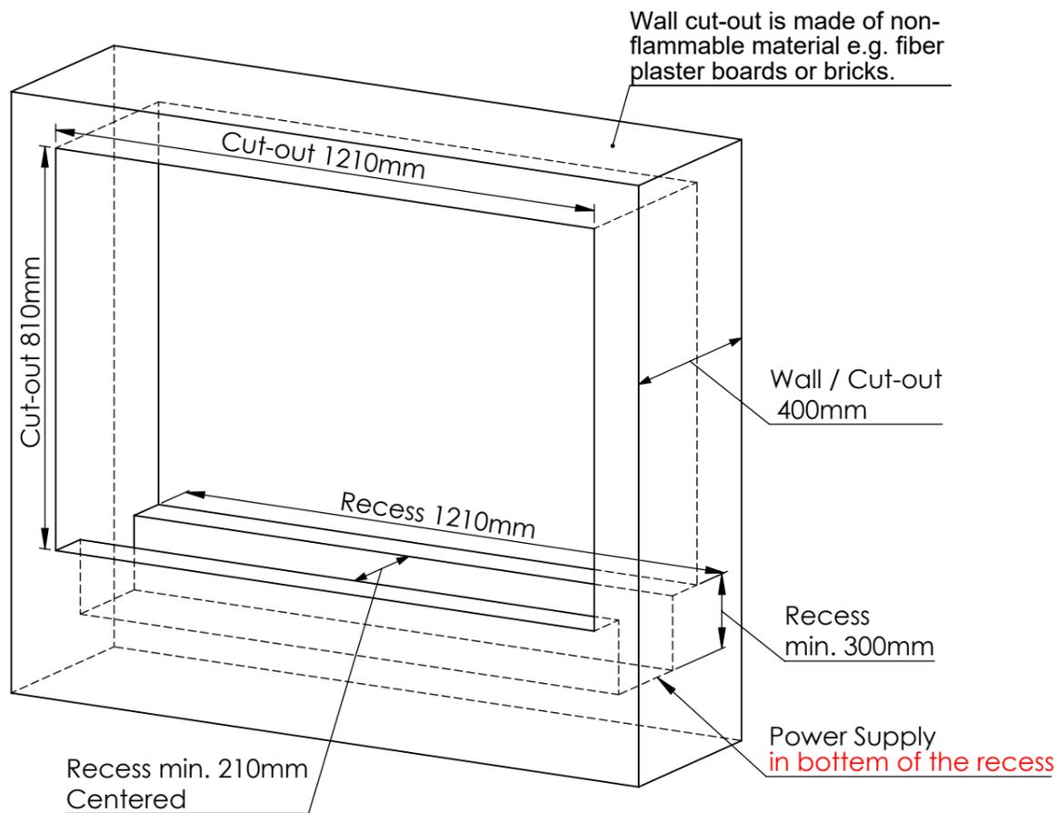
Wall cut-out is made of non-flammable material e.g. fiber plaster boards or bricks.
