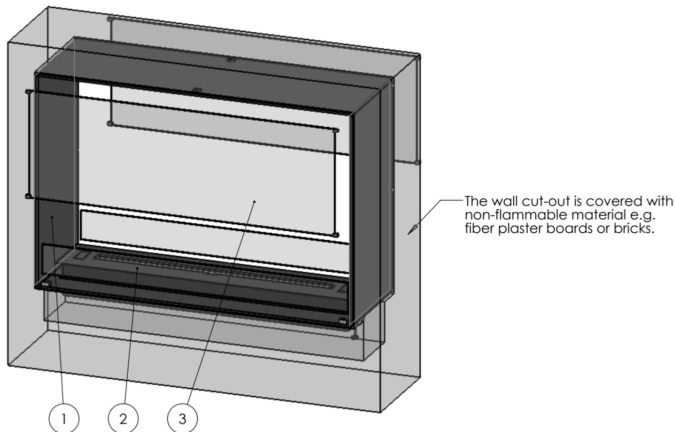
**Exploded view showing the installation process.**
